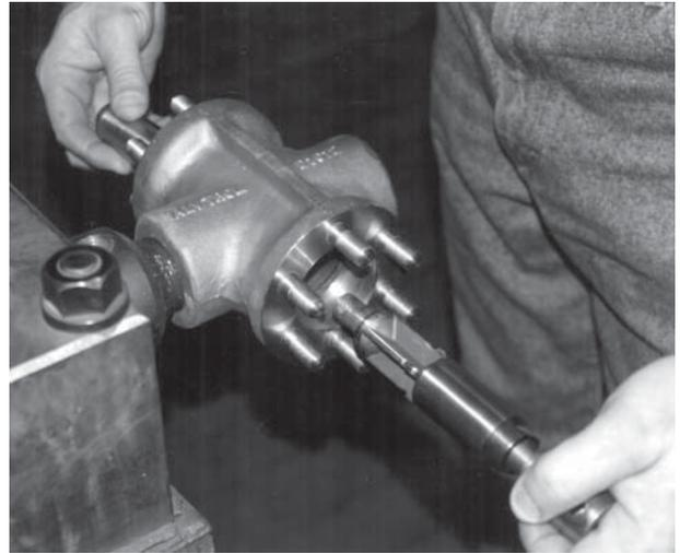
INSERT DISC AND PISTON AND SCREW TOGETHER
