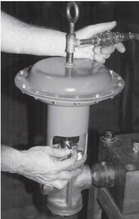
REMOVE AND INSTALL PIN WITH VALVE IN MID STROKE
