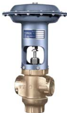
150 PSI (10 bar) Air Actuated 3-way Selector
