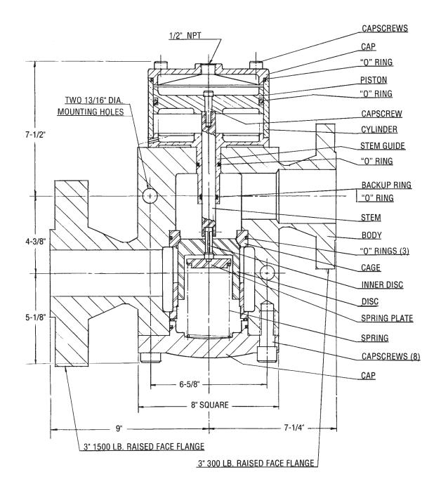
D-1260-H 3"-3,000 PSI (207 Bar) pre-fill valve shown with optional decompression feature. Give us your exact requirements so that we can recommend the proper model for you.
